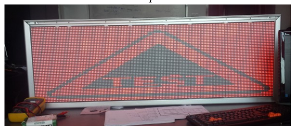
Fig.9 Image with table while displaying. In the right corner of picture is Zybo workstation
